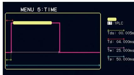
Time settings are important for pulse or sweep source. The time setting screen on the 6253 allows you to make these settings easier than the former models.
