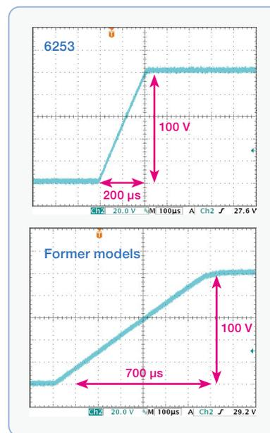
The output response of the 6253 can be switched between Fast and Slow. When the output response is set to Fast, the 6253 starts up faster than the former models.
