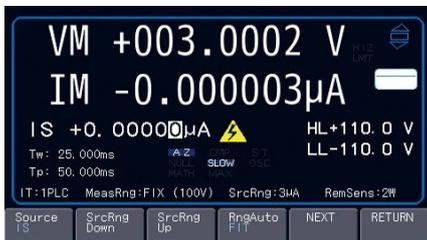
Source voltage (VS), source current (IS), limit values (HL/LL), measured voltage (VM) and measurement current (IM) are displayed. Voltage and current can be measured simultaneously.
