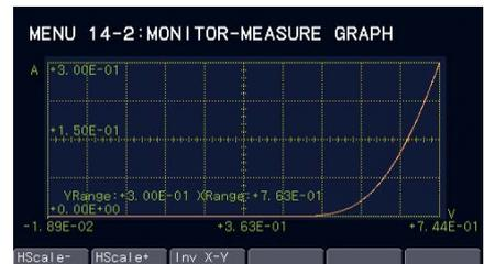
You can easily view measurement results from the graphically displayed measurement memory data.
